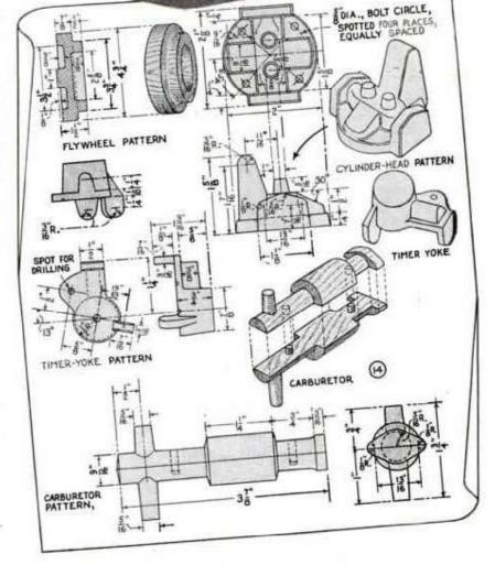
terns of this type. To make good patterns you must have good wood, of a grade suitable for pattern making. This is especially true of pine. Though the latter wood can be used, selected mahogany is always to be recommended for small patterns because of its durability, resistance to both shrinkage and expansion after working, and the ease with which it may be finished.
