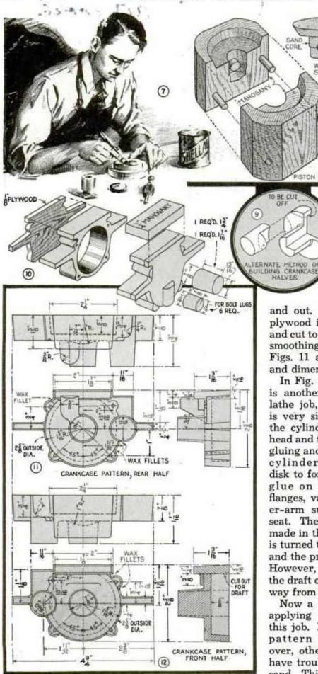
from 34-in. stock, the outer contour including the supports and bolt lugs. You can use a scroll saw, setting the blade at a slight angle to cut the draft inside
