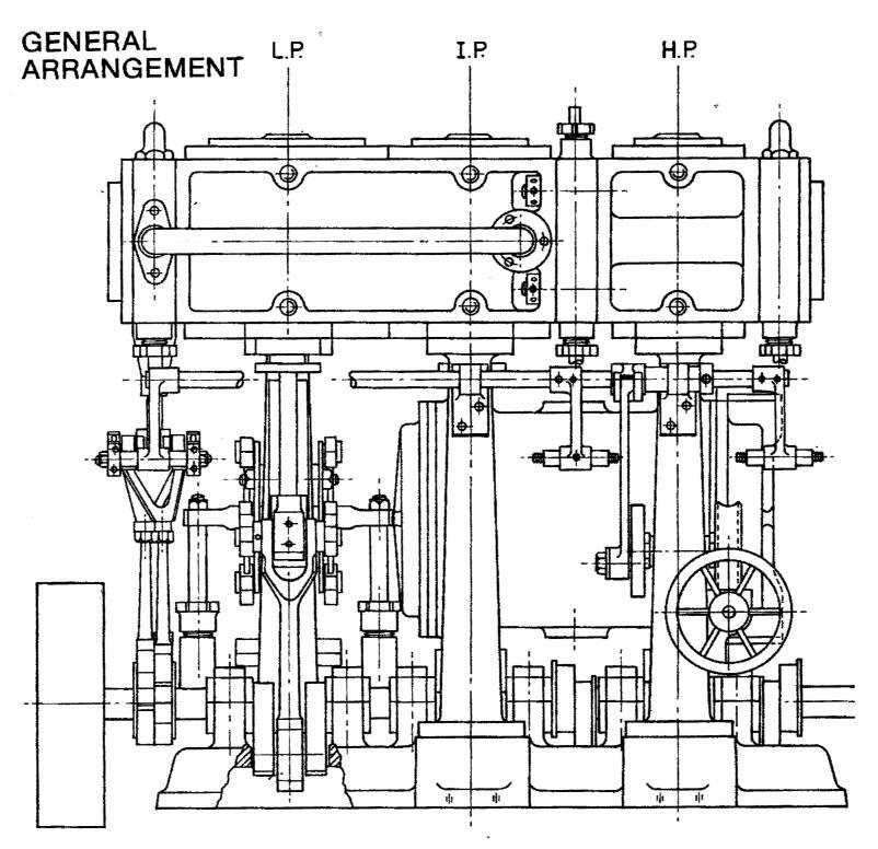
Cylinders:  $\frac{1}{4}$  in. 1 $\frac{1}{4}$  in. & 1 $\frac{3}{4}$  in. bore × 1 $\frac{1}{4}$  in. stroke
