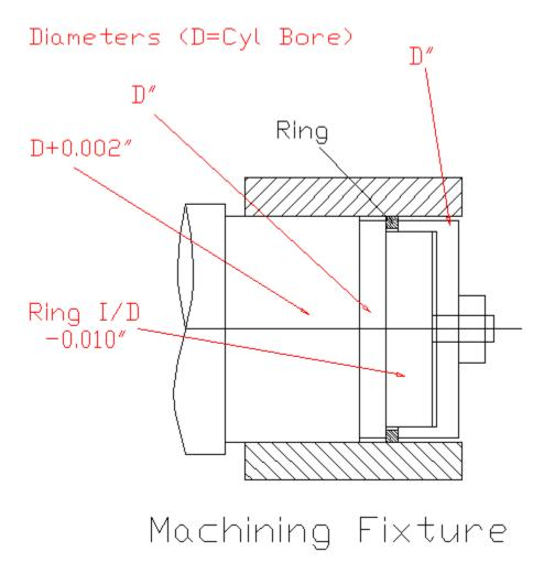
Pack the rings into the sleeve and slide the sleeve on to the rod. Fit the disc and clamp rings securely
