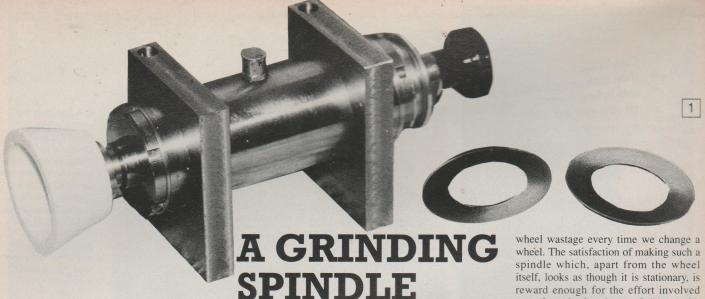
The completed grinding spindle.
