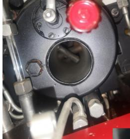
This shows the burner on Full gas (after re-jetting to get the fiercest flame possible for this application). Blow-back is caused by the excess of exhaust gas (volume) versus the restrictions of the cross-tubes and down-stream pipe. Less restriction (smaller cross-tubes?), or addition of a blower, or simply reduce the LPG gas pressure slightly with the regulator should eliminate the blow-back.
