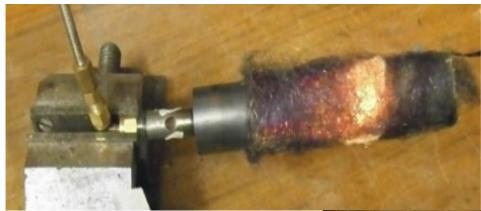
Without the radiant element the burner filled the fire-tube with flame and produced blow-back at this jet size. It was only successful with the next smaller jet. In effect the addition of the radiant element allowed more than 20% more gas to be burned in the firetube without blow-back.
