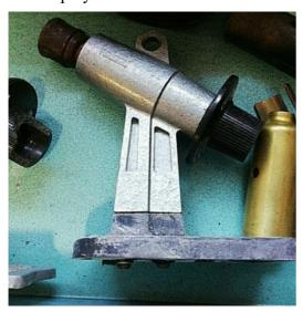
The Stephenson's Rocket burner is a valve and burner single assembly. The valve operates a needle in a jet, directly at the air intake, so a small to large flame can be achieved – from pencil flame to almost a roaring flame.
