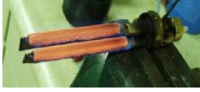
The burner tubes are covered with fine wire mesh to make a radiant element that shines on the upper half of the fire-tube. Exhaust gases disperse around the body of the burner to heat the remaining surfaces...
