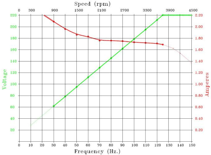
As you can see the output voltage is to all intents and purposes a straight line ending at 220.3Volts at 125Hz. If I extrapolate to zero Hertz I get my intersect at 11.74 Volts (remember my earlier estimate was 11 volts at 0Hz. And 220V at 125Hz – pretty damn close. I also expected to be 94.6V for 50Hz. – that came in at 95.2V for 50Hz. Had this been a 3-Phase motor, I could have analysed it on the VFD prior to rewinding for much better "data" rather than an experienced based "best guess".
