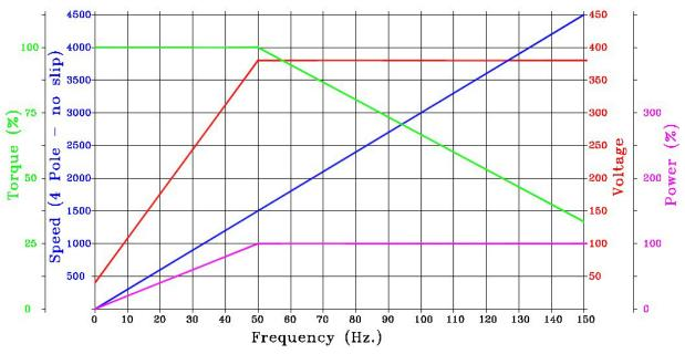
The voltage ramps up according to a **V=mF+c** function – in this case **c** (constant or starting voltage) is 40 volts at Zero Hz. Ramping up to 380 Volts at 50 Hz. (**V** being the voltage, **m** being the multiplier and **F** the frequency). (The graphics assume no slip i.e. synchronous speed is achieved – slip is normally
