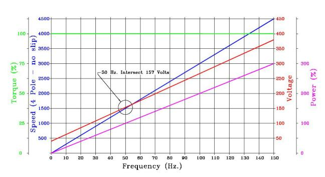
The following graphic shows the same motor but rewound for 157 Volts @ 50 Hz.
