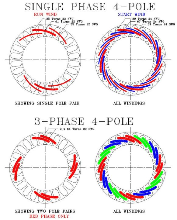
Before and after windings are as in the diagram below :-
