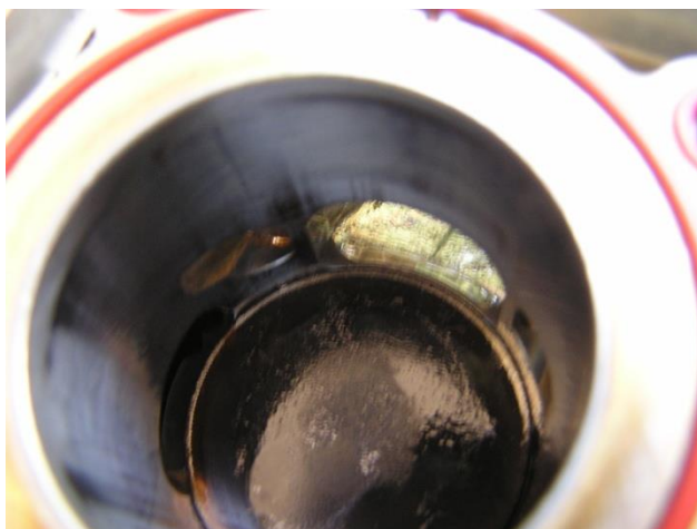
Failed CMB 35 Ringed Piston & Sleeve
