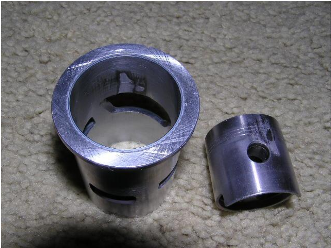
Failed AAC CMB 35 Piston & Sleeve
