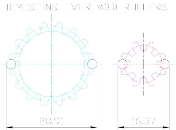
Pick a roller diameter that you have that will protrude above the teeth – offset adjacent flanks by the radius and add roller – for odd numbers of teeth you will need to use a three wire method. I use dowel pins, drill shanks and drill rod that I have to hand. Insert actual rod size into your ACAD drawing – drill shanks are typically smaller than drill size, dowels are larger than nominal and drill rod (silver steel) is normally spot on to microns undersized.
