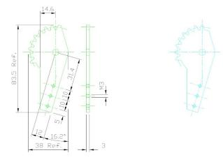
Those jaws were waterjet cut directly from the drawing data of the profile above – they meshed perfectly without any dressing or fiddling with the fit up – Eureka – it works !
