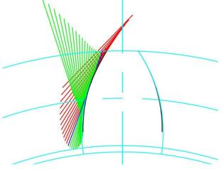
Next draw a three point arc – typically starting at the outer diameter intersect, the pitch line intersect and ending at the nearest inside line termination (black line above) vis:-
