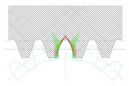
A MAAG gear shaper in fact planes gears by using a rack shaped cutter – with each cut the "rack" is advanced and the gear rotated – in so doing it generates a true involute curve.
