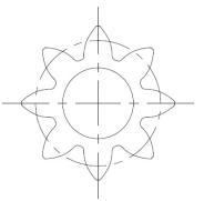
The above small pinion gear used in Slotcar racing - leaves far too little material to the Ø2.0mm driveshaft bore so the pitch circle is made larger - results in a non-standard tooth profile - but it does work.
