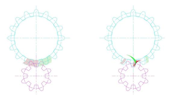
For the next profile generation we are going to do it radially -a'La a FELLOWS gear shaper where the cutter takes the form of a gear and planes the other gear in much the same way as the MAAG gear shaper only using a circular rotating cutter rather than a rack.
