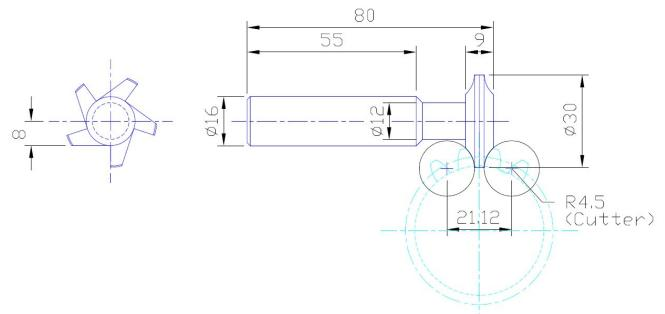
Turn the blank and in a dividing head or rotary table, mill the radii using the correctly sized cutter (Ø9 in this case) – then gash the teeth – as per dimensions determined from your drawing. Make shank to suit whatever you are going to hold it with.
