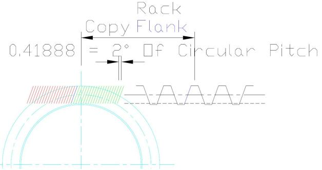
Copy a single flank (without clearance) from the middle of the rack crest to the centerline of your circular gear (In blue above).
