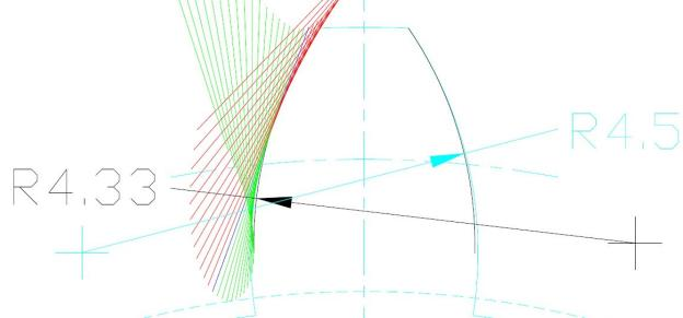
On measuring this radius I get R4.33mm – note gap – radius does not perfectly emulate involute – don't worry at this stage we will (attempt to) fix that with the pinion. Since I don't have a R4.33 cutter (although I could spin one down in a tool and cutter grinder) I go for R4.5 or Ø9.0 milling cutter that I will use to form my hob (see later).
