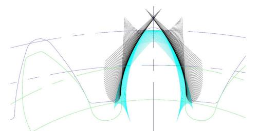
Basically a Module 2 gear profile with a 24T annulus and a 12T pinion. The resultant Ø48mm pitch circle of the annulus is therefore the stroke of the cylinder of the Hypocycloid engine.
