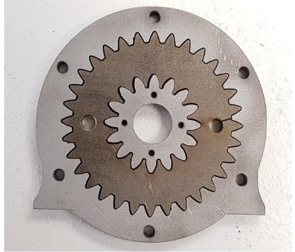
Above: The actual wire cut gear (the colour contrast is a different patina on the reverse side – so I flipped the "scrap" which makes it more visible). Link to the running engine below. Special note for EDM: The start and finish points should be in the middle of accessible tooth crests for access to "de-pip" the part – as in the above photo.
