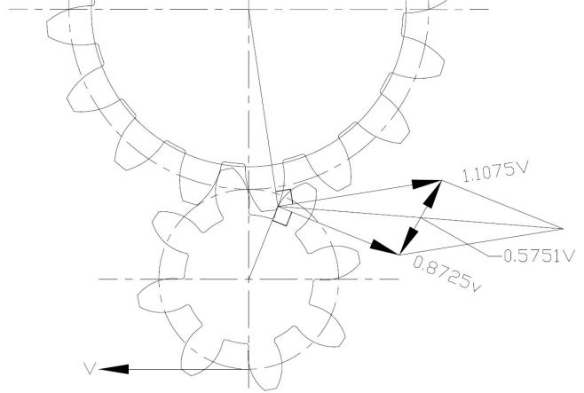
As the above vector diagram indicates the sliding velocity (at 1/2 tooth position) is as high as 57.5% of the Pitch Circle Velocity.
