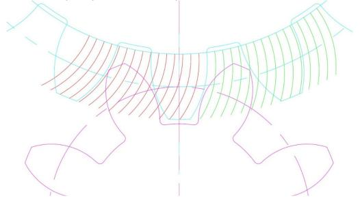
We then rotate those 4° per division (because of the 2:1 ratio) about the pinion center line vis :-
