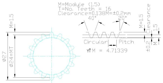
For a standard Module gear the module is the height of the tooth above and below the centerline or pitch circle diameter – in this case 1.5mm so a tooth is approximately 2xM or 3mm in this case – there is also clearance which in almost all gear calculations is 0.138M or in this case ±0.2mm.
