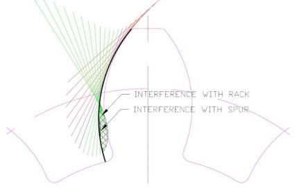
You can see why cutting with the profile of the actual spur will eliminate much of this undercutting. Since the contact between gears and/or rack is always tangential to the pitch circle, the involute shape will be the same (black line).
