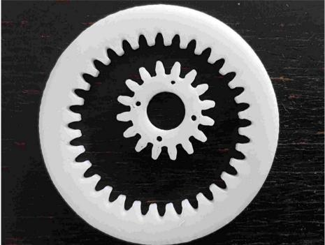
This is a 20° pressure angle – I did not like the way it fitted up – too "coggy" - and changed the design to 25°
