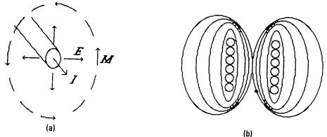
The fields around a conductor in free air: (a) field around a free wire; (b) field around a coil in free air.
