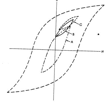
Minor loop B-H curves for various magnetic components.
