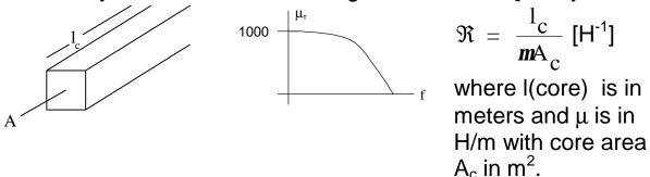
In a closed magnetic circuit as shown below  $\ensuremath{\mathfrak{R}}$  is akin to resistance.
