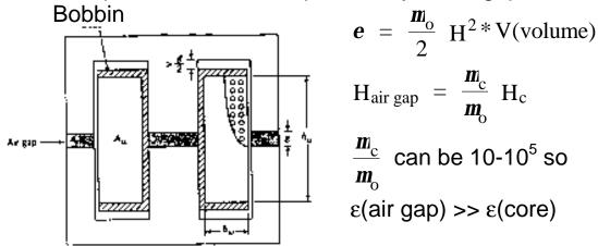
Next we compare a lossless air core inductor to an inductor made using a magnetic core.
