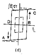
The area within the characteristic is all hysteresis loss. The only energy returned tot he electrical circuit is the thin triangular wedges above and below the saturation values.
