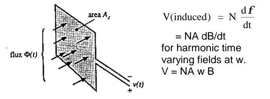
Note polarity of induced V. Using the fact that the induced B field is opposing the B field applied we can see that V(induced) causes current flow such that current out of the wire coil is from the terminal labeled +. Check by right hand rule for + current flow to create an opposing B to the applied B. We will use either V or E to represent the induced voltage.
