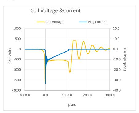
milliamps, and decreases linearly t to about 1 milliamp, at which point the arc de-stabilizes and abruptly extinguishes (which triggers the voltage ringout beginning at that point).
