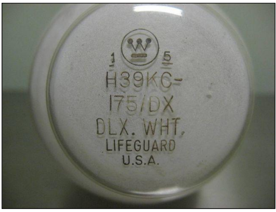
Here is a closeup of the etch of the Westinghouse lamp that came with a lot of Sylvania clearbands from eBay. The phosphor coating on the end is very thin.
