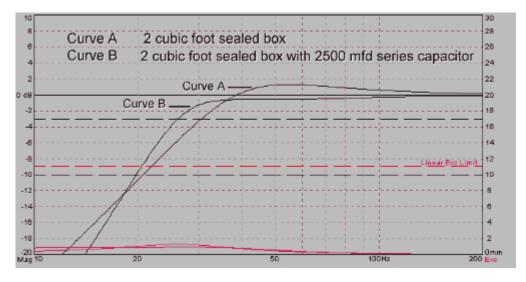
This example features an SV12 woofer in a two cubic foot enclosure. Note that the use of the series capacitor results in some loss of system efficiency. However, the curve now extends significantly lower in frequency without the peaking of the unassisted box.
