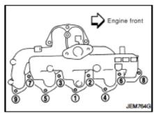
Remove intake manifold in the reverse order of that shown in the figure.
