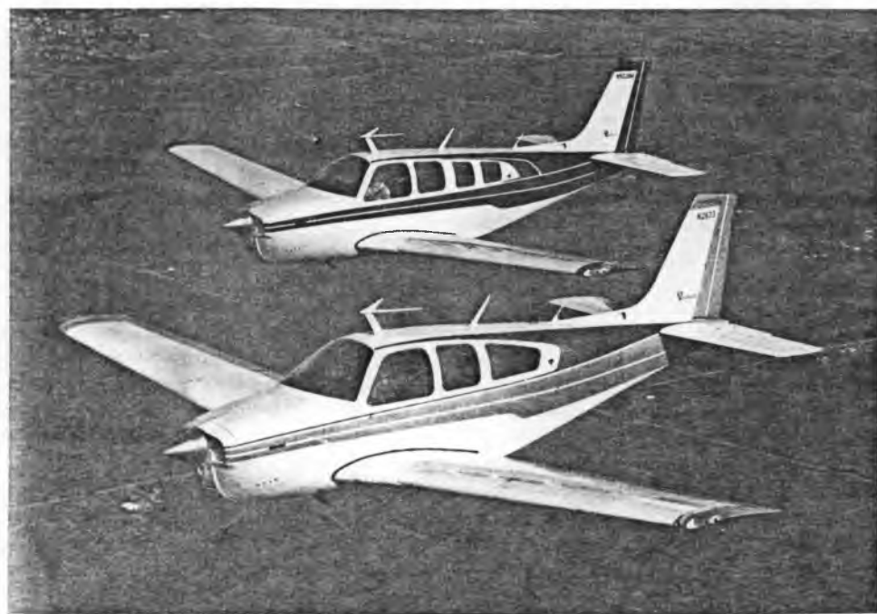
The straight-tail Bonanzas have a superb record of structural integrity—only one breakup in nearly 20 years. F33A (foreground) is virtually identical to the V35 except for the tail. A36 (rear) has stretched fuselage and higher gross weight.
