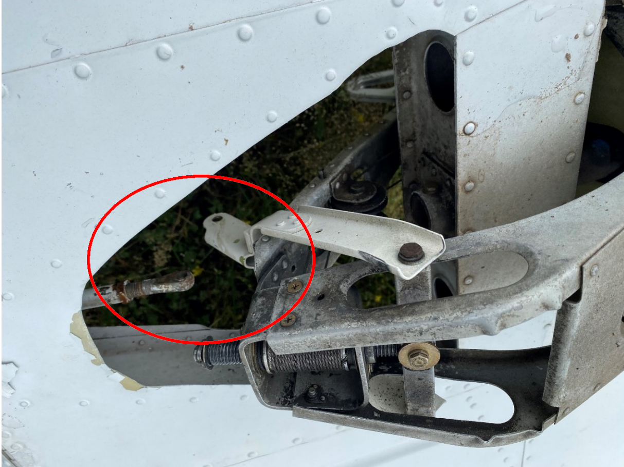
Figure 2: Photo of the stabilator trim assembly (Photo courtesy of the FAA)
