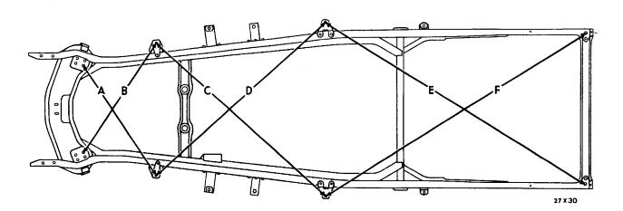
Fig. 2—Frame Diagonal Measurements
