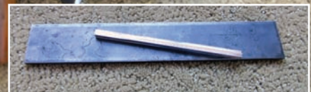
Photo 10. The pressed streamer roll after it is removed from the press.
