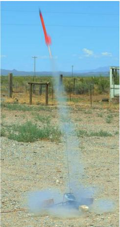
Launch #3-13.13 seconds, 64 meters. Wind gust at launch moved the tower.
