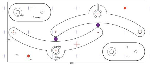
Red dots show where the clamping screws will be.
