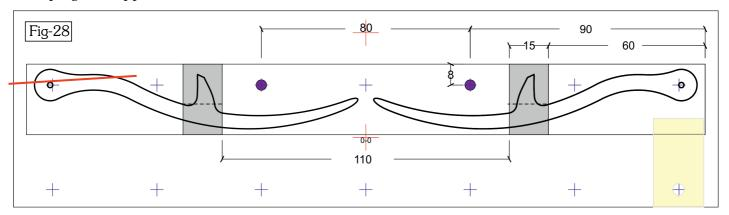
All was going well for the first two cuts around the left-hand image but on the third cut at 1.5mm deep !!! the blank couldn't stand the strain and broke away at the red line. I'll be able to cut the right-hand version out using 0.5mm deep cuts but I'll add a clamp at the bottom right corner (lemon block) as well so that may recover that.
