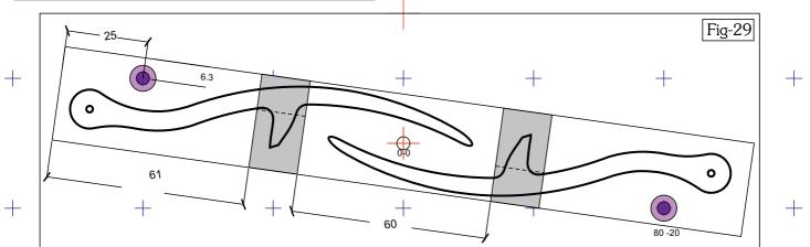
Fig-29 shows this new arrangement and will be cut from 10mm thick stock so that cutting to 8.5mm deep will retain 1.5mm throughout the base, obviating the need for tabs. It does mean that I'll have to saw the components out and machine the 1.5mm off in a second operation in the Mill (not CNC) but I have to do that for the area which has to be 6mm thick anyway.
