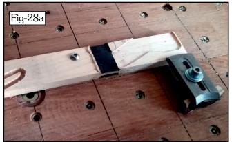
Or maybe not! — even including Tabs didn't stop the Latch breaking away during the final roughing cut. The Latch is 8mm thick at the widest part and I had a piece of Maple at 8.5mm so hoped that with 2mm 'Tabs' it would hold but regrettably not. Back to the drawing board.
