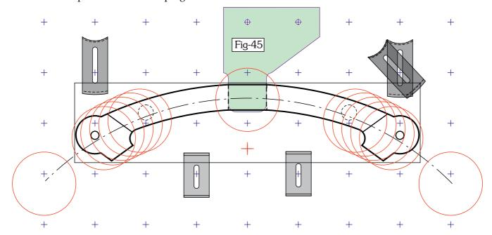
This part needs to be machined from both sides so although the centre joint is shown 'dashed' to indicate it is on the opposite side, I'll machine that first - along with the two circular recesses - and use that joint to re-position the blank to cut the end joints. That will be done by screwing a block (green - purple outline) to the table and cutting that to suit the joint, thus fixing the blank in both the X and Y axes.
