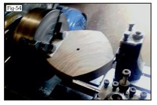
tail-stock. The centring is not hypercritical so holding a steel rule with the centre-drill and making sure the two sides are equal. Fig-55 shows this. I could have done this by checking the cross-slide dial reading for each side as well.
