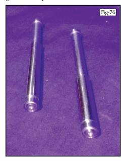
I was also aware that these small components also had quite delicate 1mm thick walls which, when assembled (glued in), would be perfectly good but in isolation may well prove an issue so I made the 'finish' cut on these parts 0.2mm. The fact that I'm using a 1mm  $\emptyset$  cutter for the finish also had a bearing on that decision!
