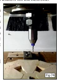
Because the drill was in place, it made sense to keep it there and change the order of operations, so, as you can see in Fig-74, the 30 holes for the Escape Wheel Pins were drilled before the Spokes or Teeth were machined.
