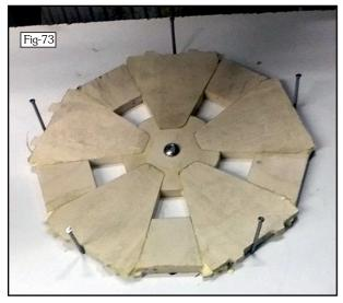
After separation and a little clean up, I found it a little challenging to get all segments to sit nicely together until I hit upon the idea to screw the centre down. Once I'd done that, the glue-up was straight forward. I was anticipating having to screw 10 blocks in a circle and add wedges to press them all to the centre but eventually was happy with just a panel pin against the end of the long segment. (Fig-73) Whether it will 'move' overnight is another matter!
