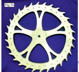
also carry the grub-screw which locks it to the spindle. The centre hole needs to be enlarged as well but these two ops were always going to be done on the lathe.
