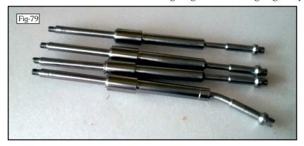
While the Denford was cutting the main 72T Drive Gear I re-made the fourth spindle.
