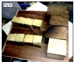
made blanks for the Winding Drum because there were oddments of Walnut, Oak and Ash laying about that were of a suitable size so Fig-81 gives you an idea of how these small items start life and Fig-82 shows the three stages that lead to the finished spacers which go between the Escape Wheel and an 8T Pinion.
