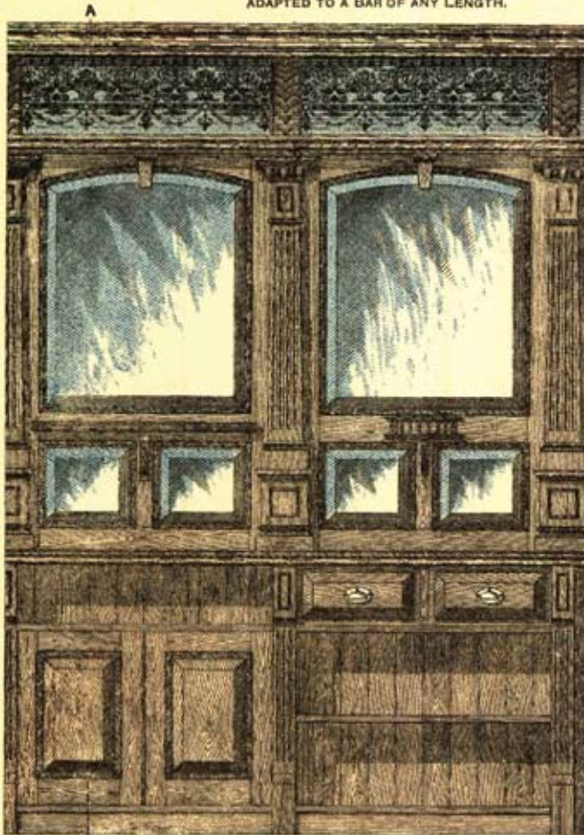
HALF ELEVATION OF BAR CABINET.
