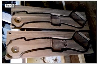
sorted the clamping out but I had to guess at the precise lateral position and although I did complete the remaining operations I won't know if the strut can really be rescued until I come to fit it to the rest of the frame. Fig-95 shows the damaged strut at the bottom and compare it with a good strut at the top. If I can make it fit then I'll still have to 'bodge' an in-fill to repair the damage. The lesson learned is that I must also clamp in the X asis.
