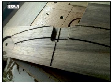
starting at 8.5mm, going to 11mm in ½mm increments. That will at least address the issue of the ribbed finish that the burr creates when using full mm pitch cuts and might stop a repeat 'rogue' cut.
