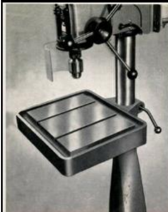
Accurately machined production table, 14 \frac{1}{2} " x 12 \frac{1}{2} " with suds trough and tee slots; optional extra on all models.
