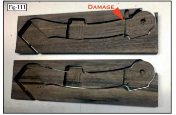
Naturally I have been investigating what might be causing this problem and have discovered that rather than the X axis motor or Ball Screw seizing up - which would be a serious issue needing difficult intervention - it seems that the X axis Stepper Motor Driver is switched off. I only found this out when I opened the back of the Denford to look at the 'Electronic' bits and in Fig-112 you can see that the middle SMD has no 'light' - therefore switched off.
