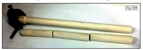
The Front Frame B sections are mostly finished but I still have to create the recesses for the Dial Pads and for that I'll have to make some positioning blocks so that I know exactly where the Dial Pegs should be.
