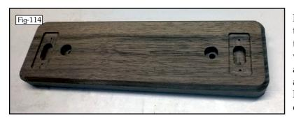
I said that there were no 'curves' on this part and that is true of my original design but when I got the first blank on the Denford I realized that it would be very easy to round the corners off and also have a pleasing chamfer following that curve as in Fig-114. To do that by hand or even on the Router Table would have been much more difficult to get right.
