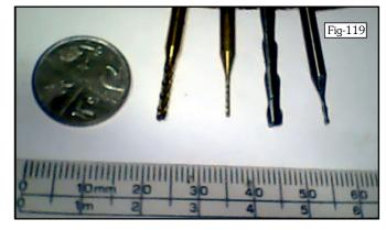
$(18 \text{mm } \varnothing)$  and a ruler marked in mm - essentially to give you a sense of scale. From Left to Right they are 2mm Burr, 0.8 mm Burr, 1/8" up-cut End Mill and 1mm up-cut End Mill. They all have a 1/8"  $\varnothing$  shank.
