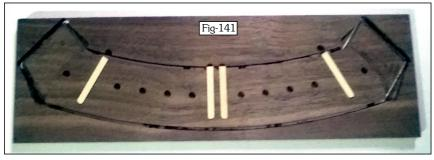
It now feels as though I'm moving forward again since I have the section C of all four Dials cut out and with Battens, Minute Dot holes and Joints all cut. Fig-141 shows the Maple Battens in place. These aren't glued in yet but I will do that on the A & E sections before I cut the joints for the reasons I mentioned on the 27th
