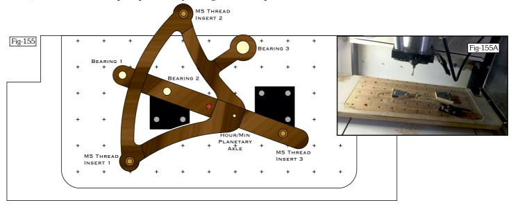
Using this set-up I could machine the three Bearings along with the Hour/Min Axle and M5 Thread Insert 3. To cut the other Thread Insert recesses I had to re-position the frame as in Fig-156 which took a little more ingenuity as far as accurate positioning is concerned. By now the Bearing recesses had been machined and I knew exactly where
