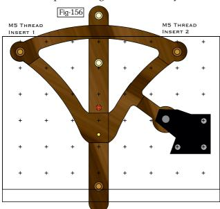
My original intention was to screw the M5 Threaded inserts directly into the frame but once I'd decided to use inserted blocks to reposition the Bearings, it became obvious that doing the same with the Inserts made more sense. It is important that Threaded Inserts are screwed into 'face' rather than 'end' grain and turning small blocks of face grain timber on a lathe has its own limitations so after making a
