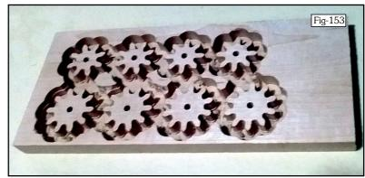
The new - slimmer leaved and smaller - Pinions are definitely better but to be absolutely sure that they will run freely I need to glue up the frames so that I can fix the locations of the bearings. The jig (read - flat board with screw blocks!) that I used to glue up the Dials was easily re-worked to apply pressure to each joint but it's a one at a time
