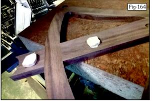
Once the Bearing recesses had been cut it only remained for me to prepare a new jig to hold the Frame perpendicular to the table so that I could cut the last two recesses for the Frame Spacers and I completed those late in the evening so tomorrow I hope to be in a position to build the basic frame.
