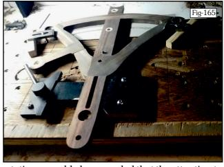
before I do any glue-up of the spacers or the Frame Brace. The tentative assembly has revealed that the attention to detail as far as using jigs has paid off since I was easily able to slide the front frame down the spacer screws bringing both frames face-to-face. I will however need to do some 'fine adjustment' to things like the Frame Brace, Bottom Frame Spacer and Vertical Adjuster block – this is not unexpected since although I'm using CNC for much of the
