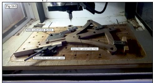
Because I needed to re-position the frames once the Maple Insert Buttons had been glued in so as to cut the Bearing recesses I did not want to disturb the side locating block but at this time I hadn't made the Maple Buttons. These buttons are 12, (14) & 18mm Ø and 6mm thick so can come out of offcuts.
