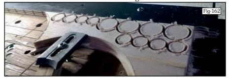
out edge because the recess and the button are cut to the same size. Up to now I've done this by hand with a 2nd Cut file, however, I suddenly had a 'light-bulb' moment and realized that it would be a simple matter to use an engraving cutter - which has a 20° relief angle (Fig-163) - to simply trim the edge, putting a small chamfer on it
