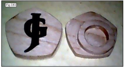
I thought that I had been meticulous with positioning the various elements (Pentagon, Circle... which are on opposite sides) accurately and also central to the blank which had to be turned over and was surprised when the surface clearing cut was about 1.5mm out. Without much thought, I made an adjustment after flipping the blank so I suspect that that was my main error.
