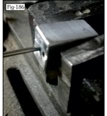
had a better idea. To hold the steel in the lathe I would have needed to cut it into shorter (600mm max) lengths and even then by the time I'd parted most of that length off there would have been a short length that could no longer be held but it occurred to me that I could drill a 14mm deep 2.1mm  $\varnothing$  hole in a block of Aluminium and use that to saw off the 120 pins I needed.
