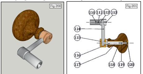
M4 thread on the bottom which would also act as a clamp for the Arm (114) - to incorporate a hexagon collar for a spanner. On further consideration I may well Drill & Tap the Arm so that the thread on the Spindle goes through it.
