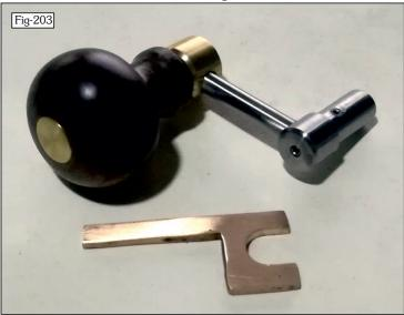
The Brass incerts proved to be simple and they are glued in place making the Knob 'captive' on its spindle so it is free to rotate but I had to make a thin 10mm A/F spanner to tighten the Knob Spindle to the Brass base.
