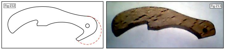
Fig-212 is the outline drawing of the Pawl and Fig-213 is the broken Pawl.
