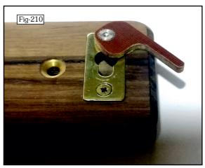
just a few tenths of a millimetre. There seems to be two ways to deal with this, either trimming the length of the screw or adding a small piece of steel or brass to the bottom of the hole.
