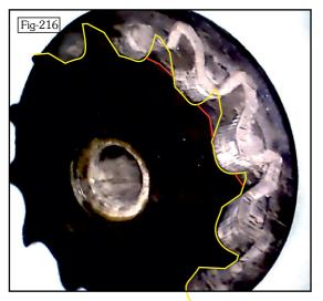
The Ratchet is already glued to the Winding Drum so affecting a repair to this is going to be fraught with issues.
