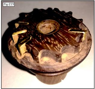
left for 10 minutes before mounting the Drum in the lathe and taking cuts of about 0.2mm soon got all the Brass Teeth at the same height as the wooden ones.
