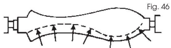
Chisel inclined in direction of cut
