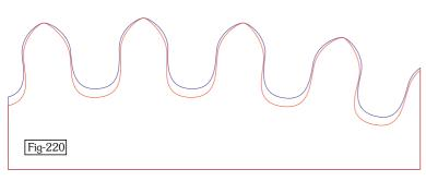
movement. I only took off 0.2mm from each tooth flank but I also cut the root 0.5mm deeper.
