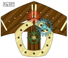
position which might have impacted upon the design of the Dial but, doing it with hindsight, it will go 50mm lower and be set inside the main Dial. This means that it is slightly more complex in-as-much-as it will need three gears rather than a direct 'pointer on the end of the Escape Spindle'.
