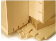
Check the fit, and take the square corners off each tail so that they fit into the rounded pockets. You don't vary the fit by raising and lowering the cutter, as with a dovetail jig, but simply track to one side or other of the line on the template. As usual the simple visual ways are best.
