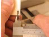
vernier (or digital) calipers. Double fraction, and remake the line of the measurement, and reset the pin-pricks. Retry the fit. calipers. Make it about 0.2mm less, as you will need room for glue in the joint and use this measurement to set your divider points.
