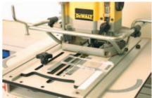
Locate the scratched line over the first pin-prick. Fix the acrylic down with Blu-tak.
