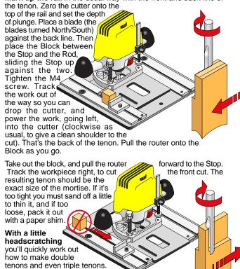
The Block will work for the double mortises as well as the tenons. **By using** a similar Block, you'll also be able to make finger joints, but that will have to wait for another WoodRat corner.
