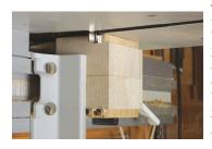
The work is cammed onto the sliding bar, and run through the cutter as a single stack. The router is brought forwards by two cutter widths each time, fixed down, and the work run through again. There are several ways to hold the work: taped or clamped up and cammed into the CamLock.
