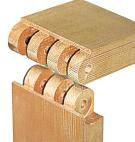
**Cut piece B in the same way.** Using the points *between* the points that you used for piece A.
